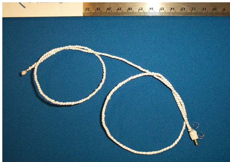
Figure 10. Photograph of a 40 W tubular AFC prototype (patent pending)
