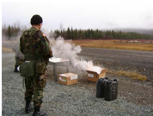
Figure 1. Activated RUSHM with steam and hydrogen gas evolution
