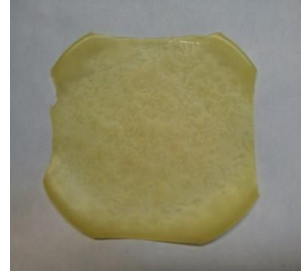
Figure 10. Photograph of IL-PVDF membrane
