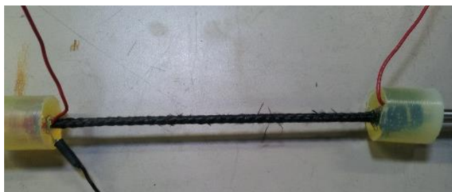
Figure 6. Photograph of Carbon Fiber Braided Tubular MEA
