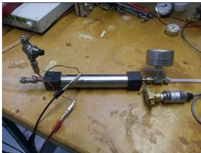
Figure 7. Photograph of a Single Tubular Reactor
