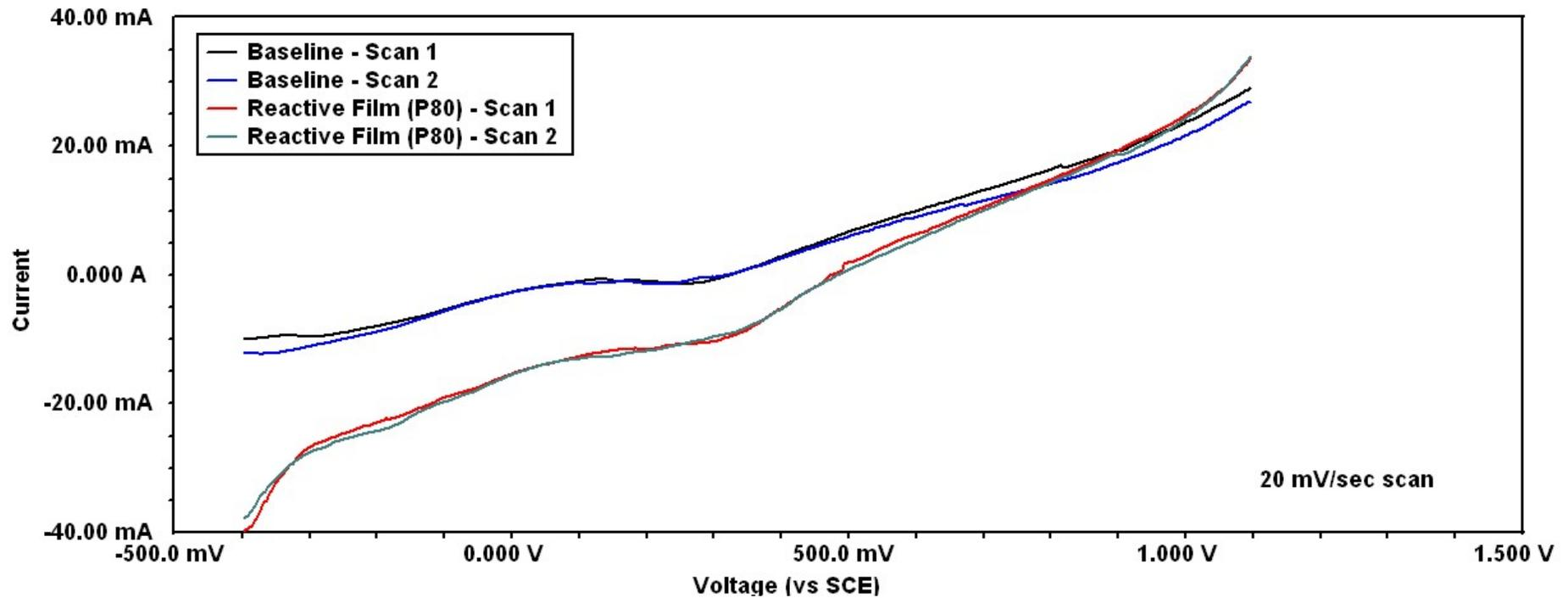
At  $-0.4$  volts, the classic “wet-electrochemistry” method gives a current density of  $41 \text{ mA/cm}^2$  whereas the sensor probe gives a current density of  $39.8 \text{ mA/cm}^2$ , a 2.9% deviation!
