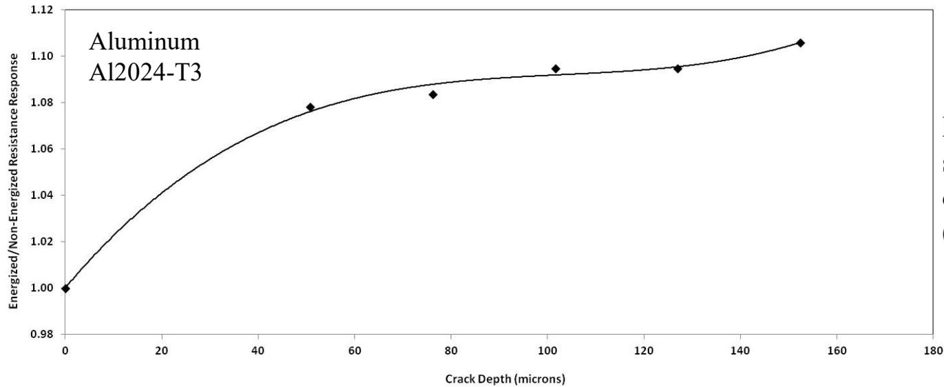
Increasing electrochemical signal up to 150 micron deep cracks (statically-induced)
