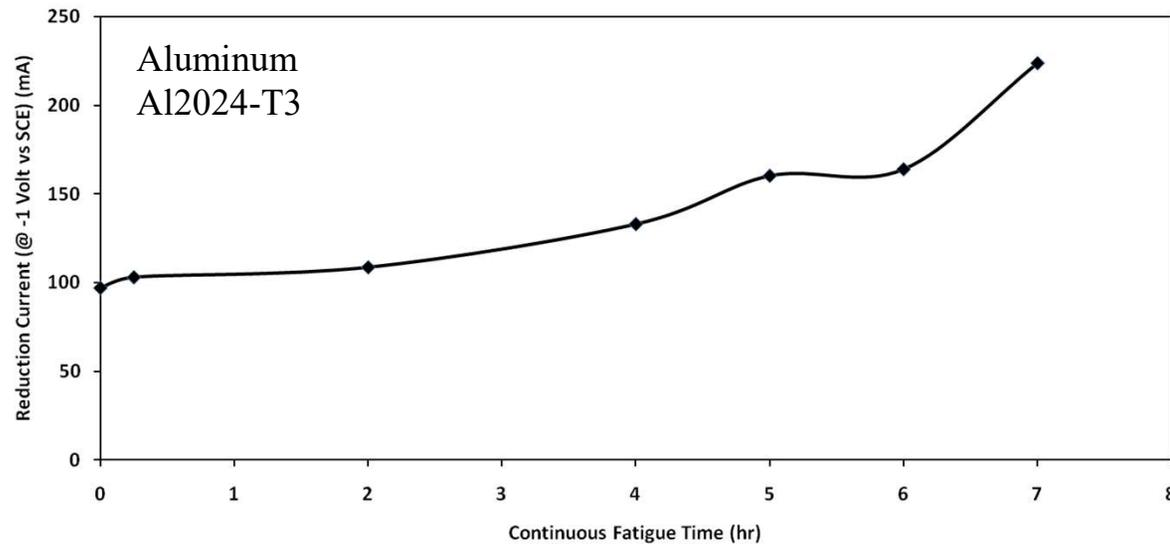
Increased electrochemical signal up to 50,000 cycles
