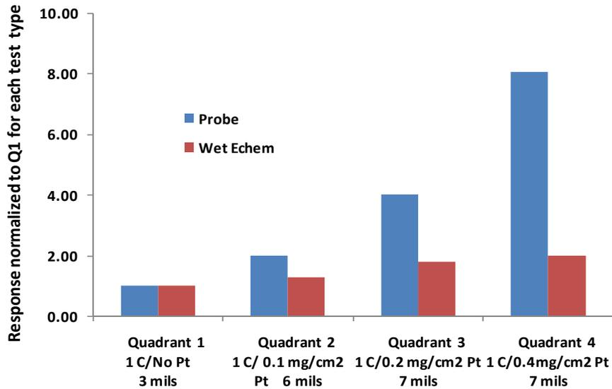
Coupon D: concentrations of 0, 0.1, 0.2 and 0.4 mg Pt/cm<sup>2</sup> over one carbon layer. Thickness is total for 1C, 0 or 1 Pt layer.
