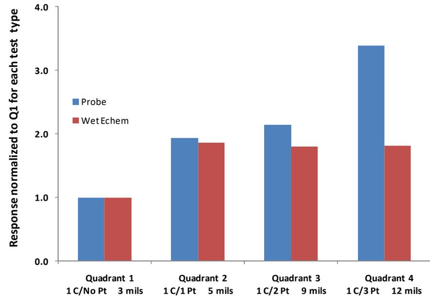
Coupon C: zero to 3 layers Pt over a single C layer
